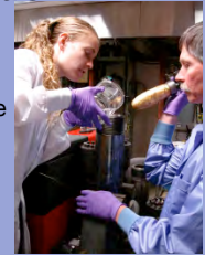
Fig 3: Bob Rosenbauer and Kaitlynn Heflin place the flexible gold cell and pressure fluid into the pressure vessel
